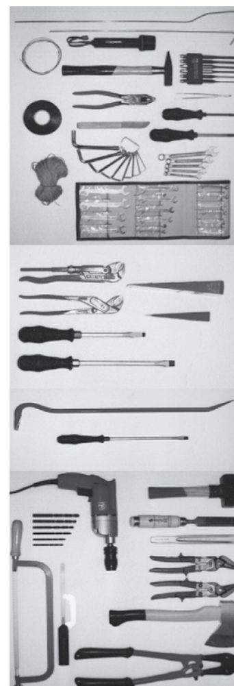
Tools used for testing 4th security class doors.
